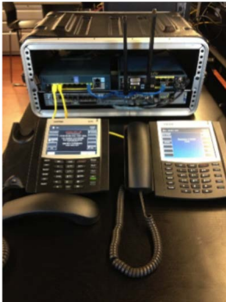
Figure 12 - above, micro MEVO disaster recovery 4g kit
